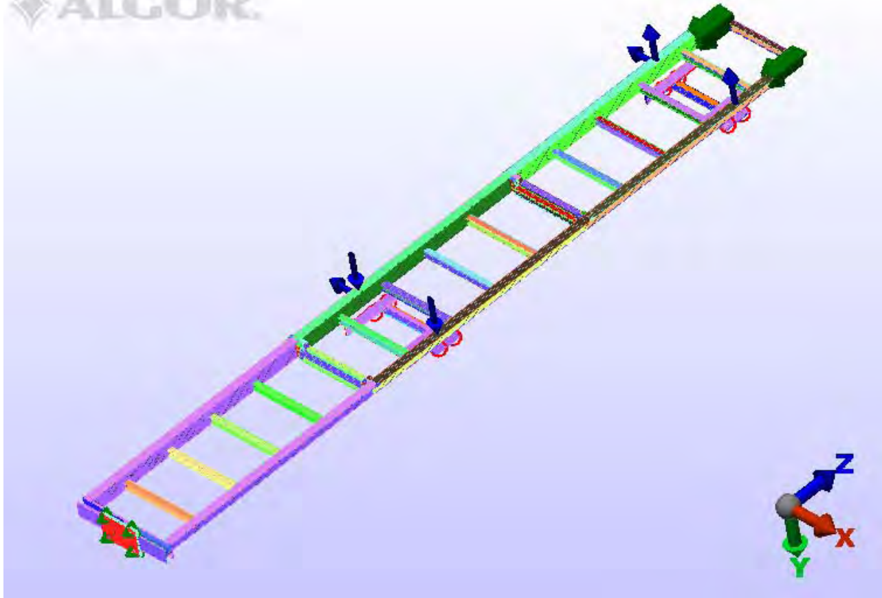
TC6K Tower Elevator Rail Assembly – Lower Three Rails Simulated Elevator Cab Loads, Lower Cab Wheels 155 Inches Above Ground Level Dead Load, Live Load, Earthquake Load, and Snow Load Combination
