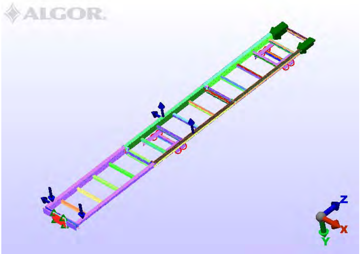
TC6K Tower Elevator Rail Assembly – Lower Three Rails Simulated Elevator Cab Loads, Lower Cab Wheels 12 Inches Above Ground Level Dead Load, Live Load, Earthquake Load, and Snow Load Combination
